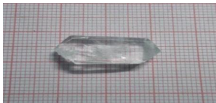
Fig. 1. Photograph of as grown LLLT single crystal
