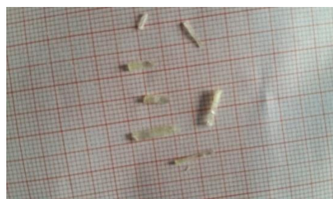
Fig. 2 Photograph of LP4NP Doped Zn 2+ single crystal
