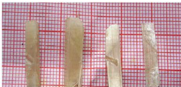
Fig.1 Photograph of pure LP4NP Single Crystal
