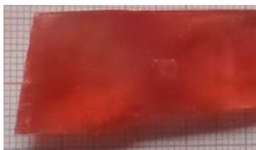
Figure 1. Xylenol Orange doped ZTS Crystal
