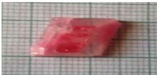
Figure1. Rhodamine-B doped BTCC Crystal
