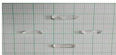
Fig. 1. Photograph of as grown LLA single crystal
